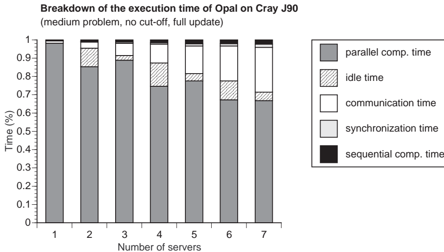
Figure 12: Breakdown of the execution time into scalable computation for different numbers of servers.
