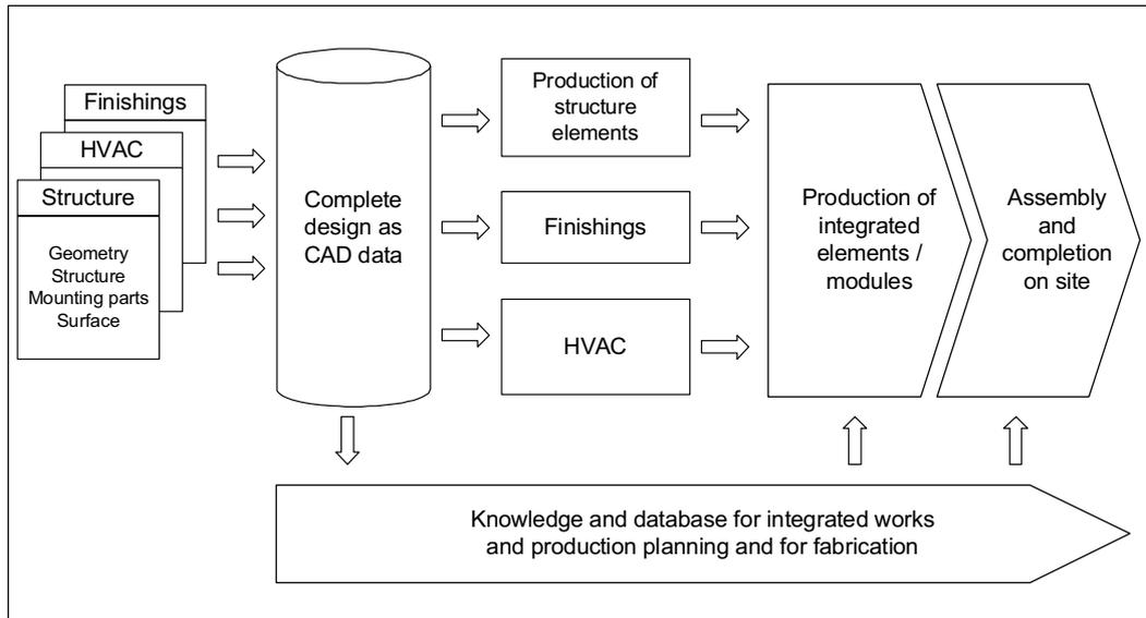
Figure 4: Structure of the planning and construction phases
