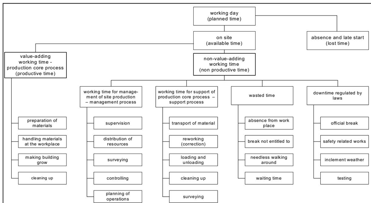
Figure 1: Systematization of working time on a construction site [14]
