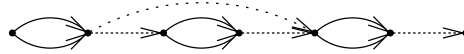
Figure 9: The contraction of the corresponding nodes (here shown for the network above) leads to three bundles of parallel edges on edges with no slack time.
