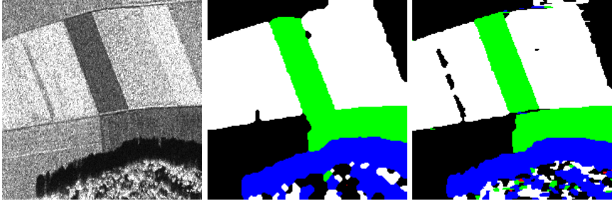
Figure 4.10: Stabilization of segmentation results by edge information for a strong smoothing constraint: Smoothed segmentation (middle), and the same experiment repeated using edge information (right), both conducted on the image in Fig. 4.4.
