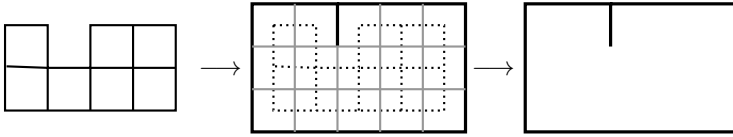
Figure 3.3: Converting a solid grid graph to a polygon.
