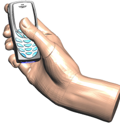
Figure 4.24: The influence of a user's hand on the mobile phone antenna performance is analyzed in data mode, that is, typing message or browsing.
