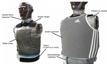
Figure 9.23: The multilayer conformal applicator in Figure 9.22 is like a vest for the treated patient. The inflated air bladder can significantly reduce the air gaps between the water bolus and a patient's skin [195].
