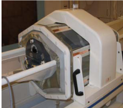
Figure 9.27: An improved design of the Sigma-60, the Sigma-60-Ellipse [201]. It has similar performance but a bigger treatment area for larger patients.
