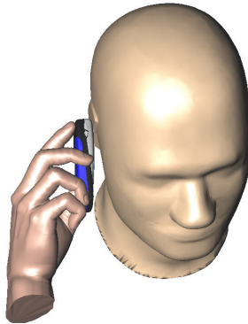
Figure 2.5: The influence of a user's hand on the mobile phone antenna performance is mainly evaluated in the talk mode
