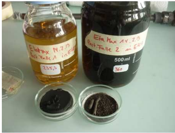
Figure 5-23: Left picture: Solid deposits and tars dissolved in ethanol withdrawn from the particle traps after experiment L1 (left: salt separator effluent, right: at back effluent). Right: Simplified scheme of the Konti-2 indicating the positions of the filters and points of withdrawal.
