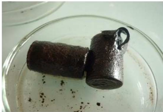
Figure 5-24: Tar deposits in filters after experiment L1; left: filters at back effluent (2), right: filter at salt separator effluent (1).
