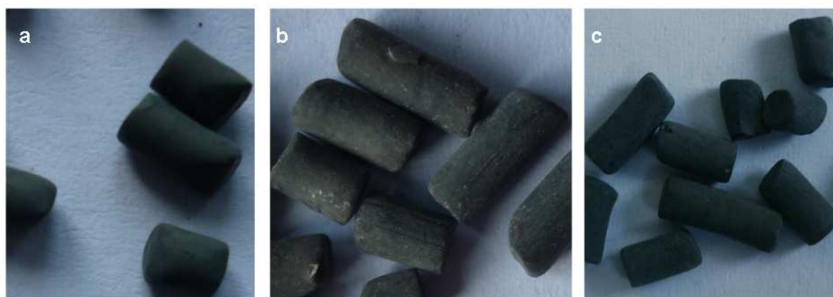
Figure 5-49: Photographies of fresh (a), used for gasification (b) and poisoned/regenerated (c) 2% Ru/TiO 2 (8) catalyst. Samples were taken from the top layer of the catalyst bed.
