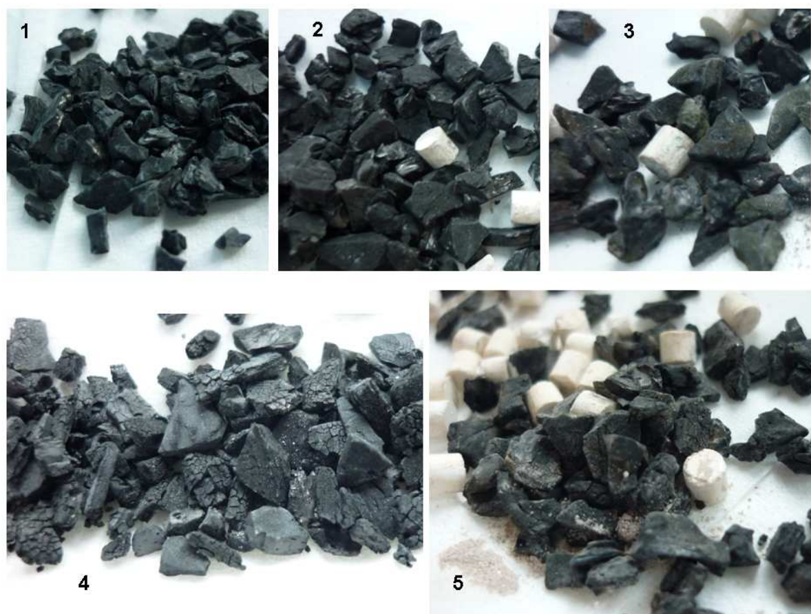
Figure 5-41: Photographs of spent catalyst samples 1-5 (see Table 5-3). Samples were taken from the top layer of the catalyst bed.
