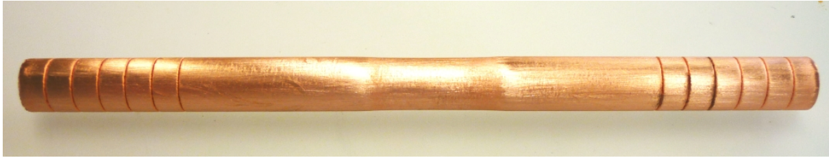
Figure 4.5: Boron carbide tube, coated with about 100 \mu\text{m} of copper. Grooves (500 \mu\text{m} deep) were cut into both ends to improve the interlocking between solder material and boron carbide.
