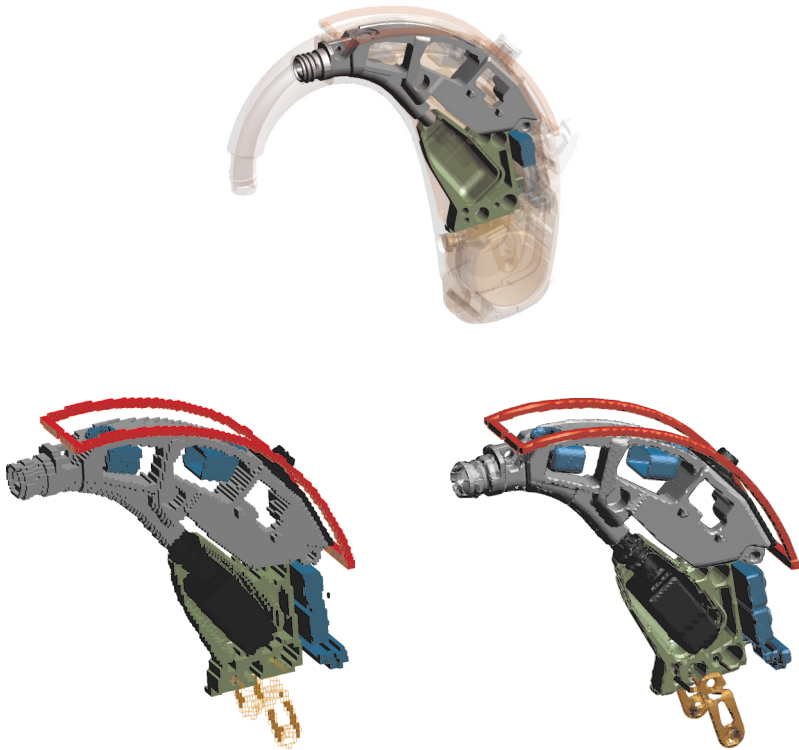
Figure 4.13: Hearing aid: 106 parts are discretized on a 201 \times 186 \times 107 grid. The parts are highly curved. Therefore, conformal simulations have to be favored.
