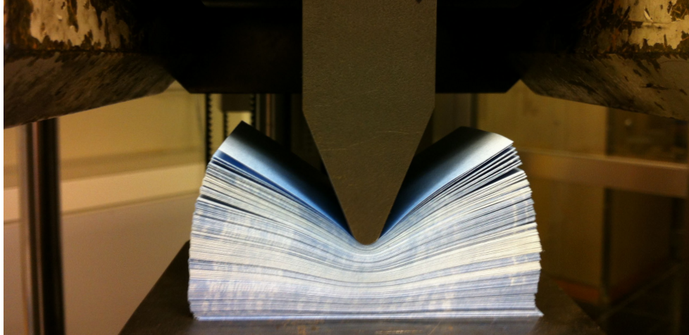
Figure 4.10: Experimental setup for determining the stack stiffness. A blunted edge (radius of 3 mm) is driven into the stack without cutting any sheets.
