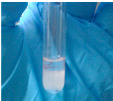
Figure 7.2: Octanol saliva mixture. Mixing Octanol with saliva formed stable droplets that formed a third, milky phase between the saliva and the octanol phase. The picture was taken 11 days after mixing.
