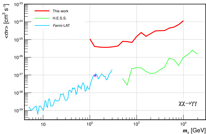
Figure 15. Upper limits on \langle\sigma_{\text{ann}}v\rangle for direct DM annihilation into two photons, from the Segue 1 observations with MAGIC (red line), compared with the exclusion curves from the GC region observations from Fermi -LAT (3.7 years, blue line, [62]) and H.E.S.S. (112 hours, green line, [63]). Also shown is the \langle\sigma_{\text{ann}}v\rangle value corresponding to the 130 GeV gamma-ray line (violet triangle, [64]).
