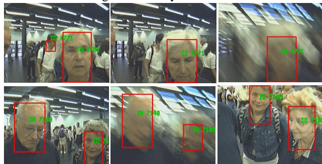
Figure 5: Visitors at the Expo.02 seen by the robot. Skin colored regions show a light border. Dark borders indicate clusters that passed the heuristic filters. The face tracking algorithm is able to maintain the visitor Ids even with a moving camera and resulting out of focus images.
