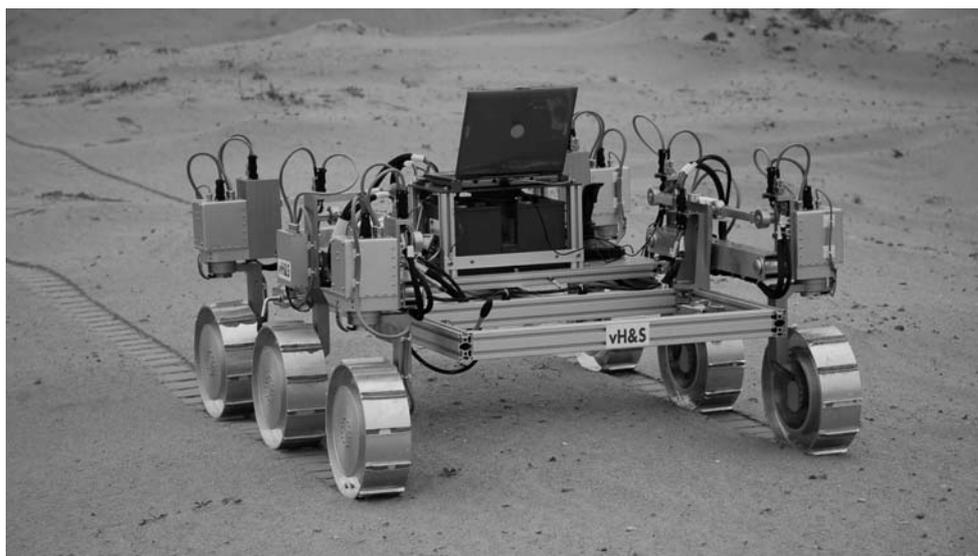
Figure 1 Exomars Breadboard Rover Chassis (a.k.a. Bridget)
