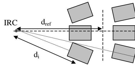
The use of such a steering method has consequences on the wheel speeds. They have to be proportional to the distance  $d_i$  to minimize slippage.
