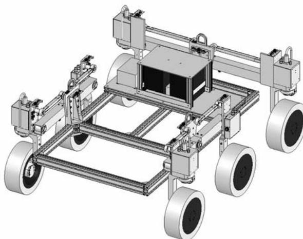
Figure 2 CAD model of breadboard design (RCL-E)
