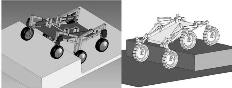
Figure 3 (left) CRAB chassis, (right) Exomander (RCL-D) Chassis
