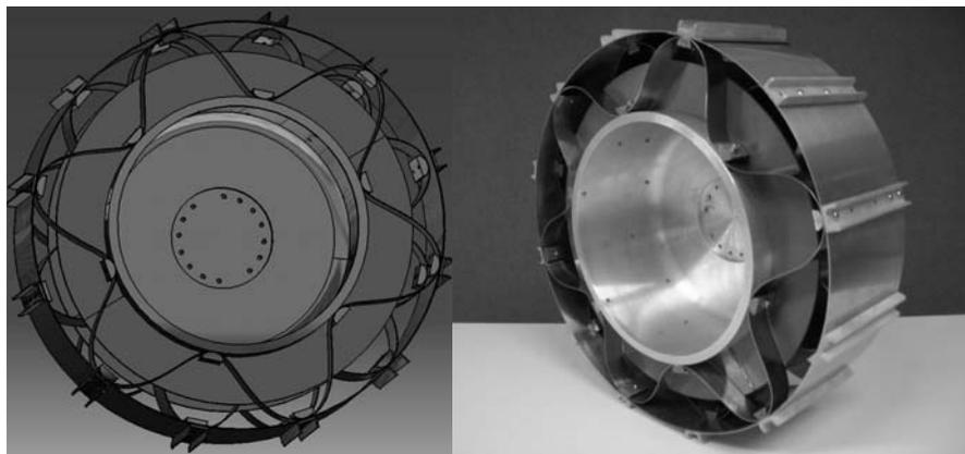
Figure 5 Flexible wheel: CAD model (left) and as manufactured (right)
