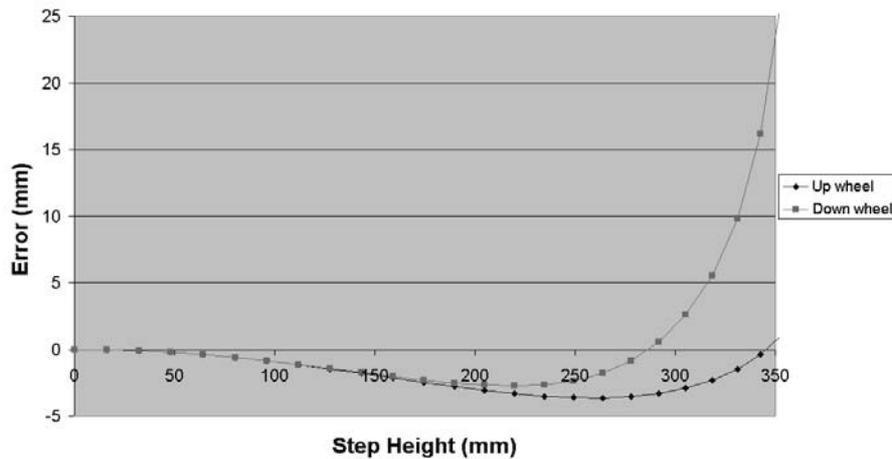
Figure 4 Horizontal Displacement versus step height (vertical difference between each wheel)
