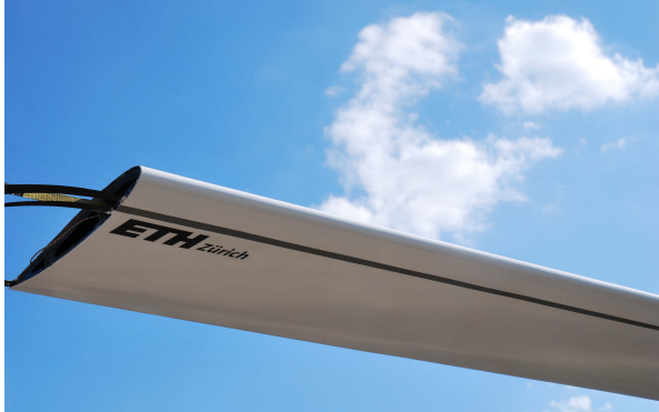
Figure 4.51: Completed experimental airfoil structure based on thermomechanical coupling
