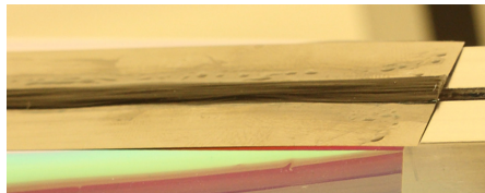
Figure 5.10: Local reinforcement of the electrode of the experimental wing box structure by carbon fibre roving
