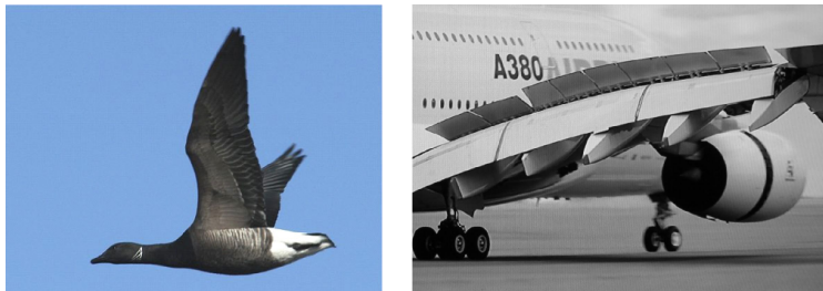
Figure 1.2: Examples for the difference in shape adaptivity of birds and state-of-the-art airplanes: Brant goose ( Branta bernicla ) during flight [5] contrasted with flaps and ailerons of an Airbus A380 [6]
