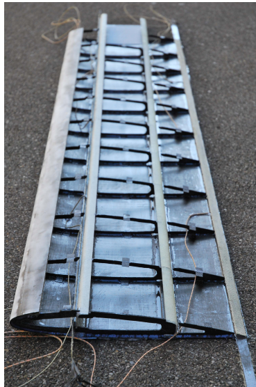
Figure 4.50: Inner structure of experimental airfoil based on thermomechanical coupling
