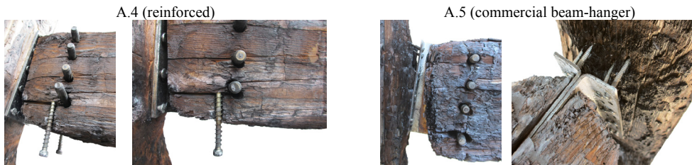
Figure 8. Connections A.4 and A.5 after the fire tests.
