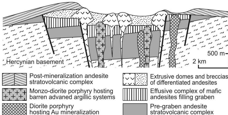
**Figure 1.** Simplified section of the Javorie stratovolcano hosting porphyry gold systems in a central volcanotectonic graben zone (adapted from Konečný et al., 1998).
