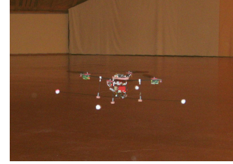
Fig. 4. OS4 in hover. A training frame was added for safety.
