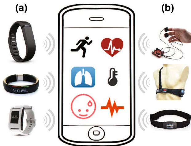
Fig. 7 Different types of sensors in external wearable devices: a physical sensors are used for tracking of physical activity; b bio-physiological sensors measure biological activity of the human body such as galvanic skin response, respiration or heart rate
