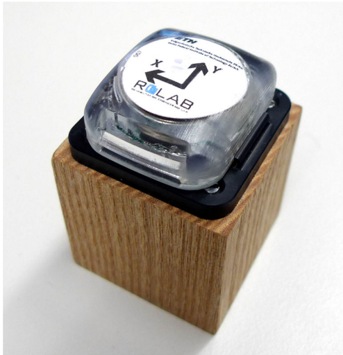
Fig. 2 A ReSense sensor module attached to the calibration cube for manual calibration
