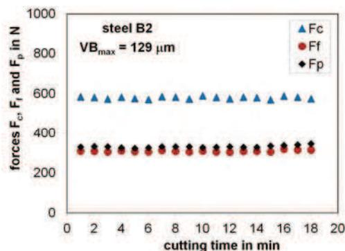
Figure 5 Evolution of  $F_c$ ,  $F_f$  and  $F_p$  for steel B2 under improved machining conditions
