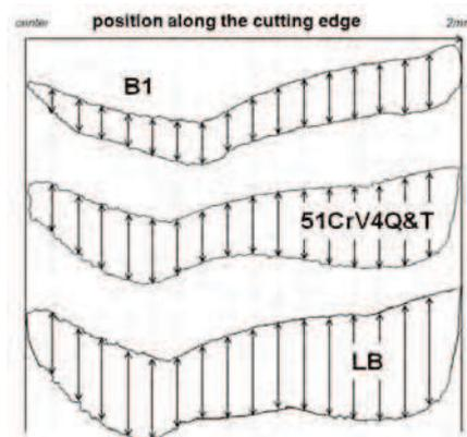
Figure 2 Chip thickness across the  $\varnothing 4$  mm-drilling tool
