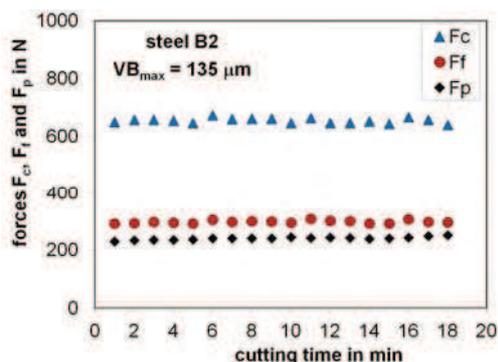
Figure 3 Evolution of  $F_c$ ,  $F_f$  and  $F_p$  for steel B2
