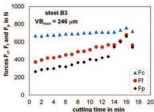
Figure 4 Evolution of  $F_c$ ,  $F_f$  and  $F_p$  for steel B3
