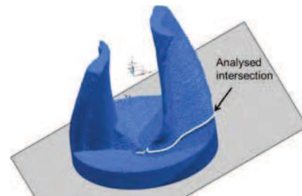
Figure 1 CAD reconstruction of chip root
