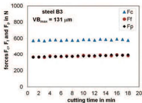
Figure 6 Evolution of  $F_c$ ,  $F_f$  and  $F_p$  for steel B3 under improved machining conditions
