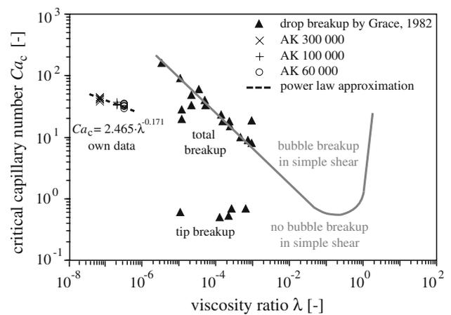
**Fig. 9** Bubble breakup in simple shear obtained in the transparent concentric cylinder device. Data for air bubbles are compared to data from Grace for droplets (Grace 1982) (*lines* are to guide the eye)
