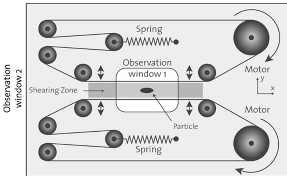
band apparatus are, in particular, higher achievable Capillary numbers even though gap width is larger and fixed (higher shear rate, four times lower surface tension of silicone oil).
