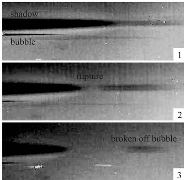
**Fig. 8** Tip breakup in simple shear obtained in the transparent concentric cylinder device. In each picture, the *upper object* is the shadow of the bubble, the *lower* one the bubble itself. Breakup can be observed more easily by looking at the *shadow* due to its 2-D projection nature (air bubble in silicone oil AK 60000, viscosity ratio  $\lambda = 3.09 \times 10^{-7}$ ,  $Ca_c = 32$ )
