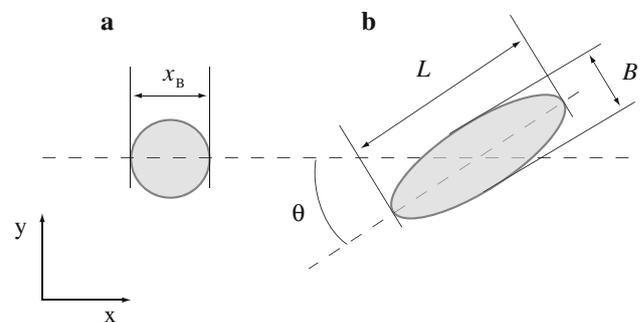
**Fig. 1** Parameters describing droplet and bubble deformation:  $x_B$  droplet or bubble diameter,  $L$  major axis,  $B$  minor axis,  $\theta$  rotation angle. **a** Initial, undeformed droplet or bubble shape and **b** deformed droplet or bubble
