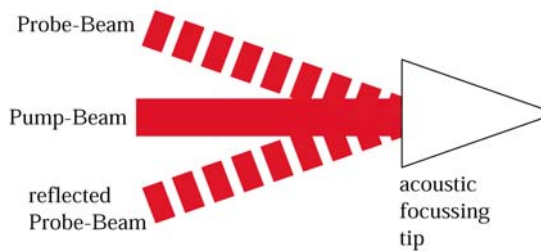
Figure 4.36 Scheme of the focusing tip acting as an acoustic lens
