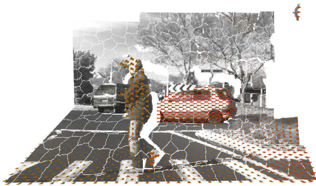
Fig. 1 Example scene from Vaudrey et al. (2008): jointly estimated 3D geometry, 3D motion vectors, and superpixel boundaries, rendered from a different viewpoint
