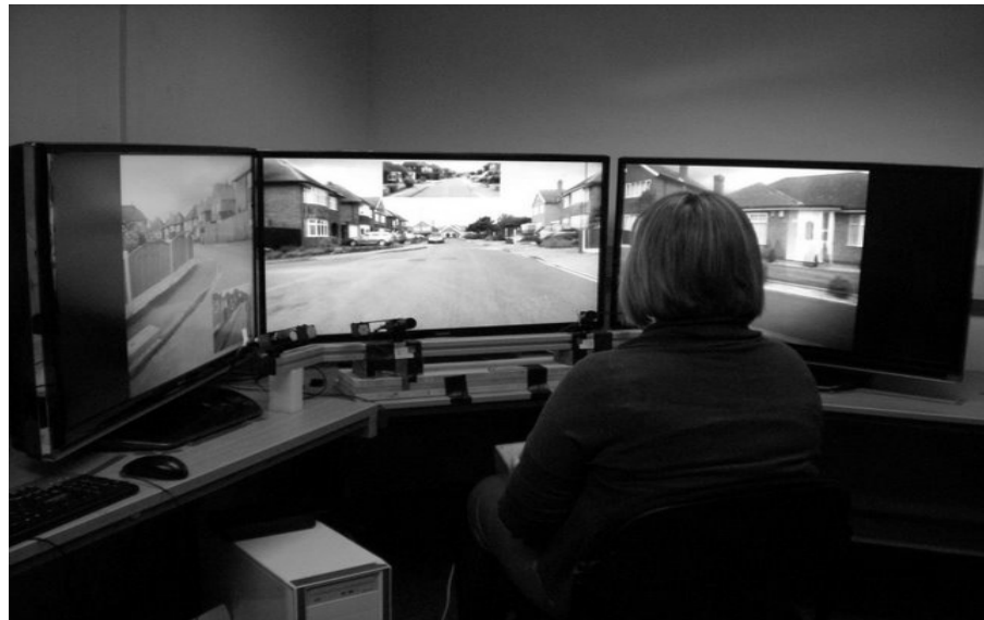
Figure 9.13: The three-screen hazard perception rig in the laboratory
