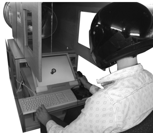
Figure 9.1: Photograph of the measurement set-up, with approximate subject positioning in front of the wind tunnel, typical clothing, and the computer screen, keyboard, and joystick used for the simultaneous VTT and AVT tests.
