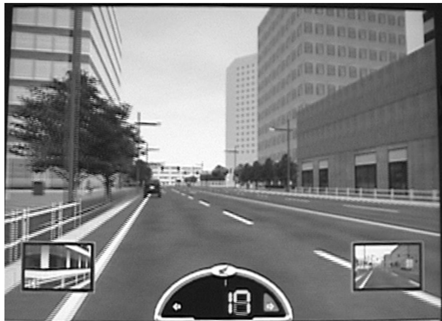
Figure 9.10: The motorcycle simulator screen (presented at approximately 3 x 2 metres)
