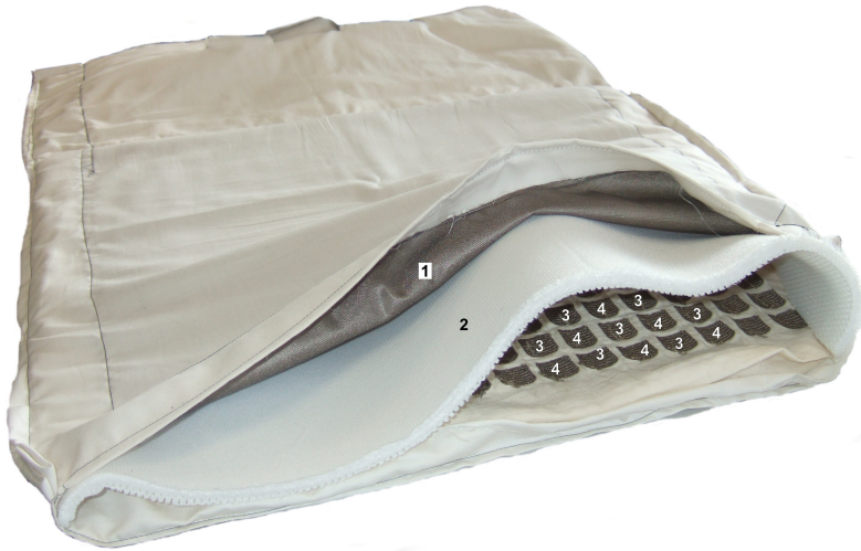
Figure 6.1. Textile sensor with 240 elements used for sitting posture measurement. 1: Common electrode, 2: Spacer, 3: Sensing electrodes, 4: Grounded electrodes
