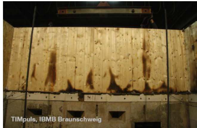
Figure 4: Previously encapsulated cross-laminated timber (CLT) surface after a parametric fire test in a compartment [16]
