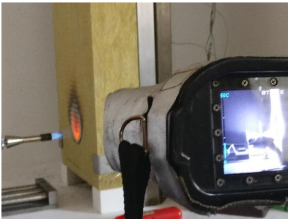
Figure 5: Initial phase of the European smouldering test EN 16733
