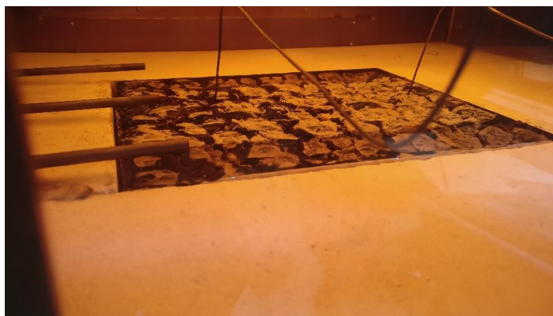
Figure 4. Installed specimen (FH03) during the exposure with surface thermocouples and the three fixed installed Pitot-tubes to measure the static pressure changes near the specimen surface.
