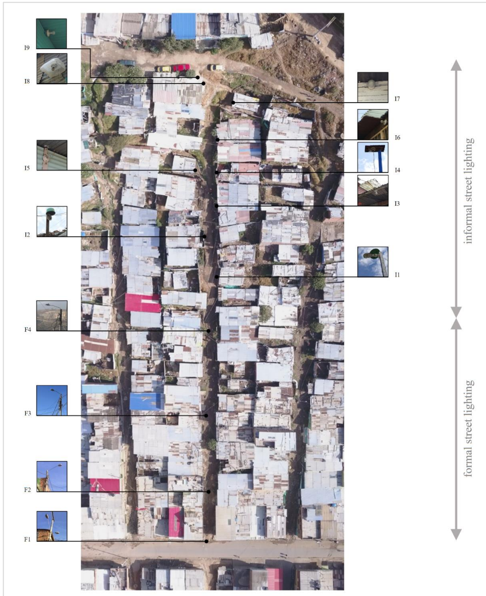
Figure 2. The Case-Study Street in Caracolí, Lit by Four Formal High-Pressure Sodium Street Luminaires Provided by the Municipality (F1-F4) and Nine Informal Street Luminaires Provided by the Residents (I1-I9)
