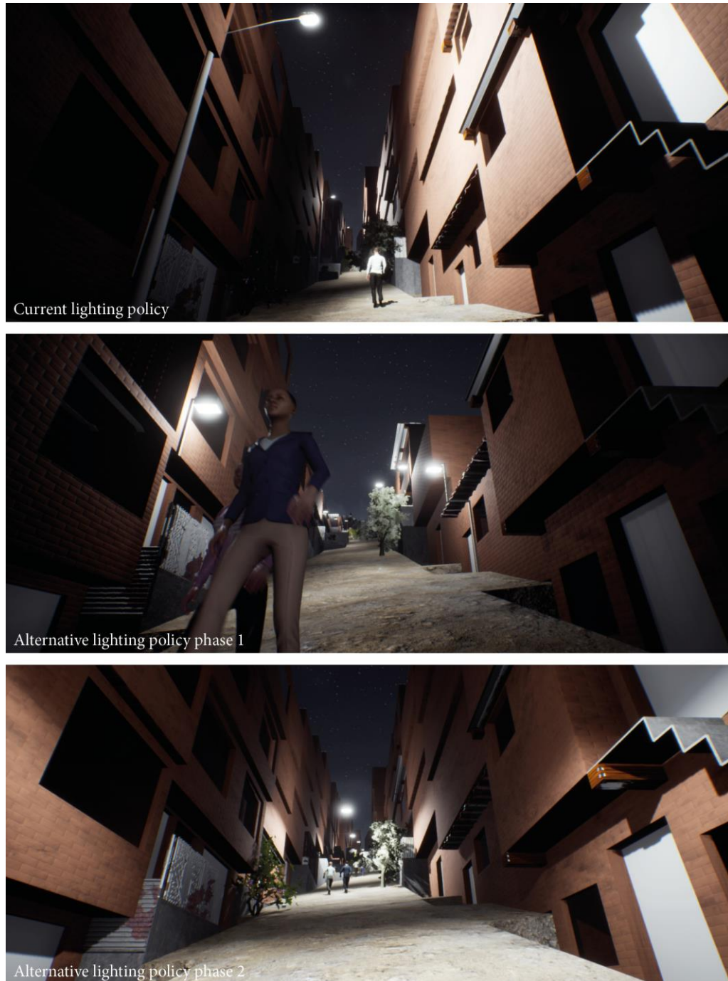
Figure 13. Scenario-Based Decision-Making Visualisation for a Multitude of Different Options, in this Case the Current Lighting Approach in the Case-Study Street as a ‘Seven-Metre-Wide Street with Four Storeys Scenario’, versus the Two-Phase Alternative Lighting Approach. All of the Scenarios Include Temporal Data such as Densification and Footfall . Visual Inspection Illustrates not only the Lighting Effect, but also Enables Detection of how the Light Column Collides with the Fourth Storey (see figure on ‘Current lighting policy’).
