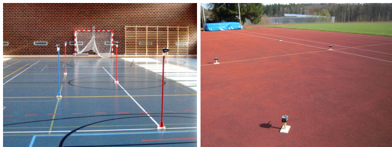
Figure 7.12: Setup of the two testbeds for the experimental evaluation of the SpiderBat platform: The indoor testbed is located in a gym, where four nodes are placed in an area of 10 \times 6 m, approximately 1.5 m above ground (left). The outdoor testbed is located on a sports ground, where we placed four nodes in an area of 10 \times 5 m, approximately 20 cm above ground (right).
