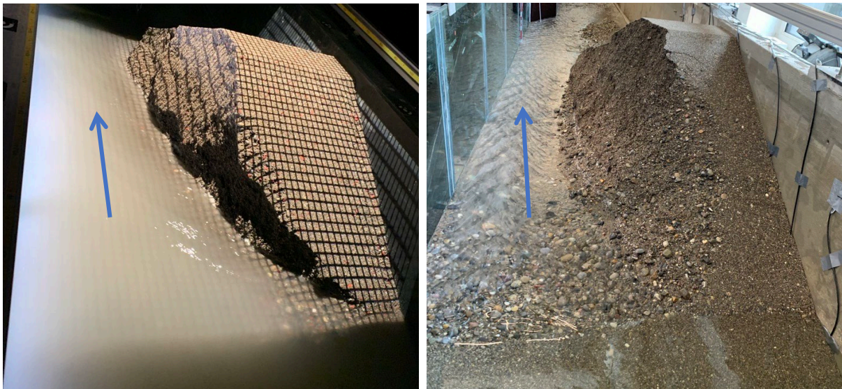
Figure 1. Medium (left) and large scale (right) laboratory experiments (after breaching). Blue arrows show flow direction.
