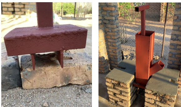
Figure 5. Stomping tool (left) and pre-crusher with inserted stomping tool (right).
