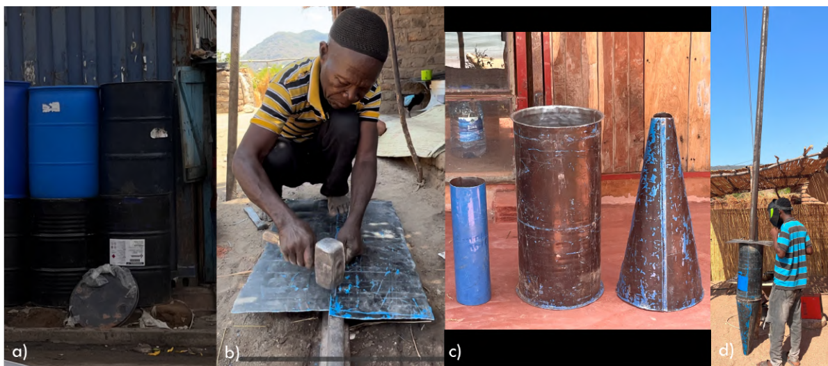
Figure 10. Four steps of the cyclone separator production: a) Empty oil drums at the market in Blantyre; b) Drum cutting and piece assembly; c) Pieces produced from the drum; d) Welding of all parts and painting.
