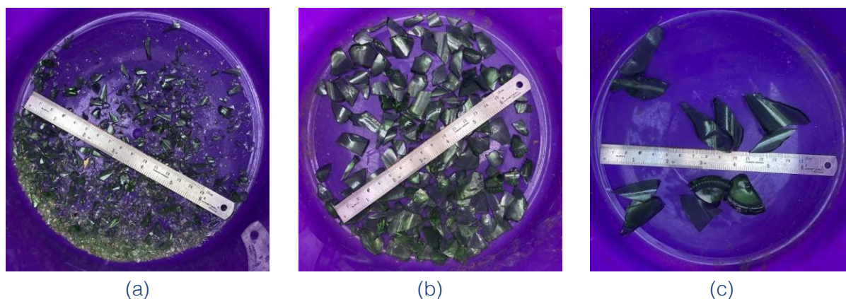
Figure 8. Crushed glass sorted by size from small (a) to large (c) with 15 cm ruler for scale.
