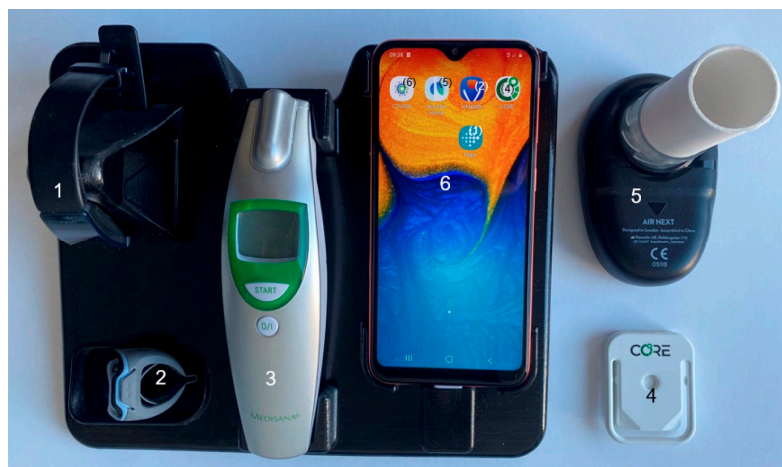
Figure 2. The COVIDA desk setup for the usability study contains a collection of sensors and monitoring modalities. Items in the picture are numbered and explained: (1) Wrist-worn accelerometer and heart rate sensor on magnetic charging interface; (2) finger ring pulse oximeter for continuous measurement of heart rate and oxygenation saturation; (3) infrared thermometer for forehead temperature measurement; (4) continuous core body temperature measurement device; (5) spirometer with mouthpiece for measurement of lung function; and (6) smartphone with daily questionnaire in the COVIDA app. The respective applications on the smartphone screen are indicated in brackets.
