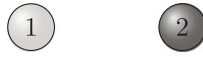
FIGURE 3 A dimer made of two symmetrical resonators. The alternate color emphasize the occurrence of the dipole mode [-11]^T
