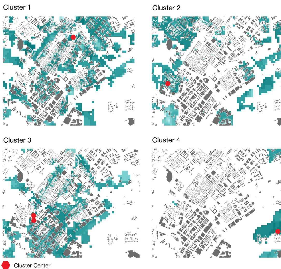
Figure 10. Distribution of the grid cells in the real two-dimensional space grouped in the four different clusters (i.e., urban settings) that form the neighborhood of Rochor, Singapore. The color intensity indicates the representativeness degree. Grid cells colored more intensely represent better the urban parameters of their corresponding clusters. The most representative grid cells of each cluster (highest value(s)) are marked in red as the candidate locations for fixed air quality stations. The gray areas correspond to buildings.
