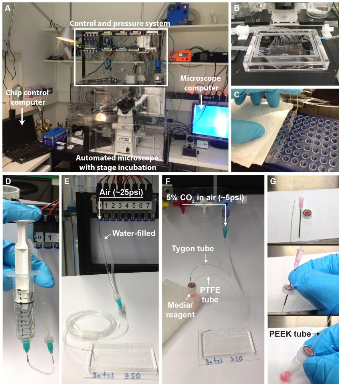
FIG 2. Photos of microfluidic cell culture system setup. (A) System overview. Solenoid valves that pressurize on-chip valves are controlled by a USB controller box operated by a laptop computer. An air pressure source is connected to solenoid valves (required pressure ~20–30 psi). The valve control system and computer are portable for use on different microscopes. A separate computer controls a fully motorized inverted fluorescence microscope (pictured: Nikon Ti-Eclipse). The microscope contains an incubation system to control temperature, humidity, and CO 2 . (B) The chip is secured tightly to the microscope stage using a stage plate with a viewing area sufficiently large to see chambers and surrounding fluidic circuitry on chip. Slots in stage cover allow tubing connections to the chip, and tubing is secured using plastic stage clips. (C) Cell retrieval from chip. A ~10-cm length section of PEEK tubing is connected to either the upper or lower waste outlet on
