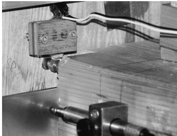
Figure 4.4: FSR pressure sensor at the connection interface
