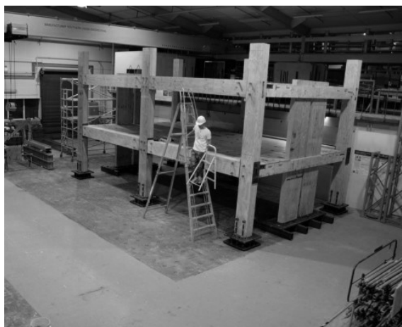
Figure 2.3: Tests performed on a scaled post-tensioned timber frame building [30]
