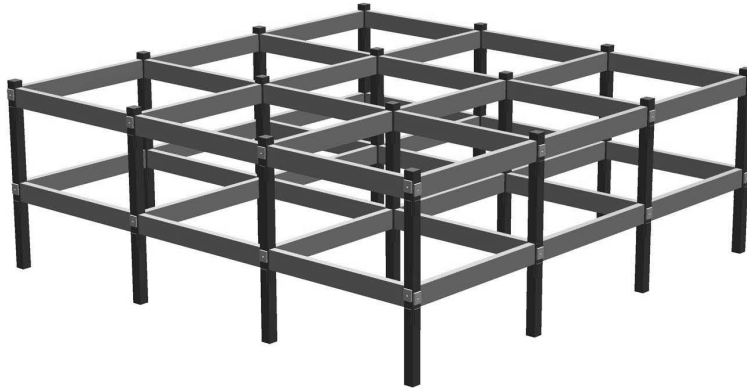
Figure 8.2: Post-tensioned timber frame in the “ETH House of Natural Resources”
