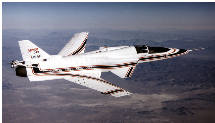
Fig. 4. X-29 experimental aircraft. The forward-swept wings configuration of the X-29 makes the design of robust feedback control systems more difficult compared to more conventional aircraft. (Courtesy of NASA)
