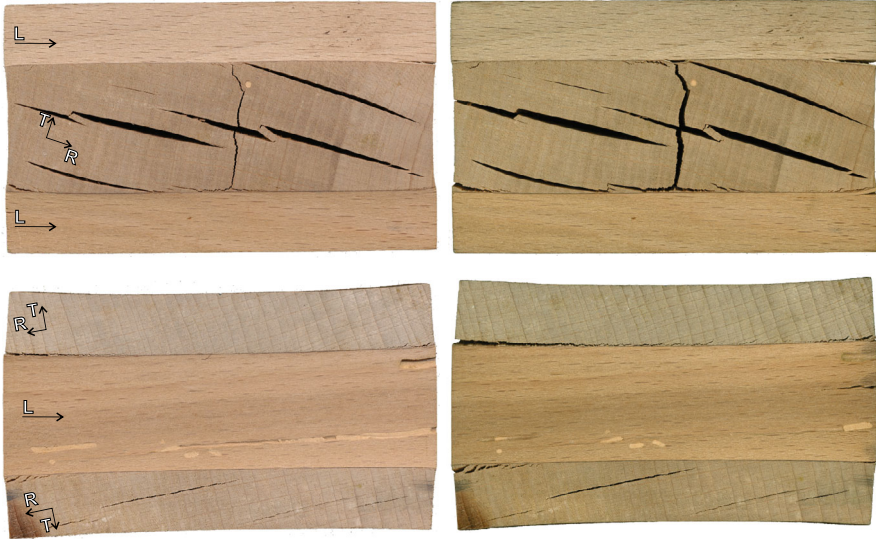
Fig. 8 Side views of the fractured P2-PUR-T4-1 sample after the first ( left ) and the second ( right ) de-moistening steps with a single straight transverse micro-crack and severe intra-laminar TL-cracking
