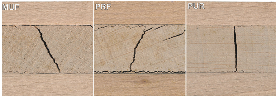
Fig. 9 P2-X-T3 samples ( d = 20 mm) with different adhesives after the first de-moistening exhibiting adhesive failure in the MUF and interphase failure in the PRF and PUR bond lines
