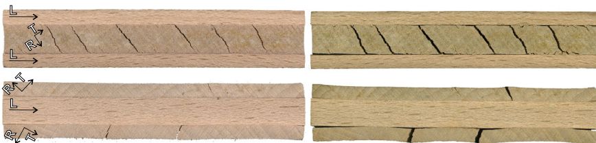
Fig. 6 Side views of the fractured P2-MUF-T2-2 sample after the first ( left ) and the second ( right ) de-moistening steps, displaying the formation of equally distanced curved micro-cracks that span the entire sample width and micro-crack-induced de-bonding
