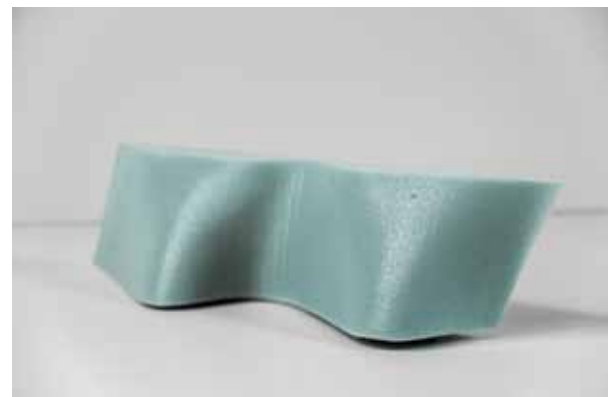
Sample wall geometry - one of two components, which are individually cut by the robot and glued to comprise one complete wall element
