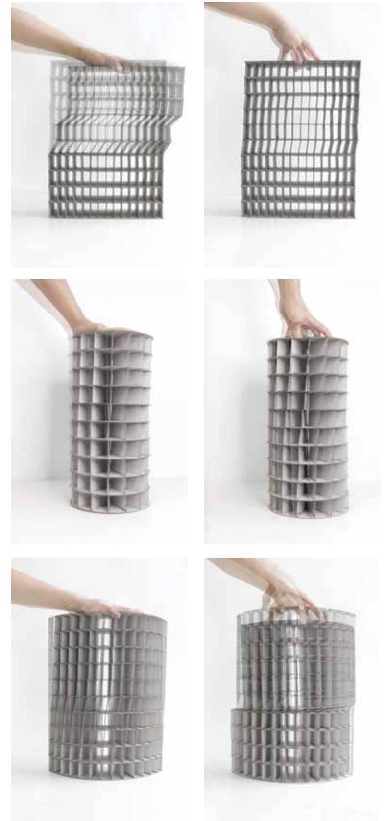
Tower 1 Multiple connected and curved open shapes turned out to be the optimal solution, combining the behaviours of the previous two models (above). Tower 1 consists of 1.200 wall elements and measures 1.6 metres in height.
