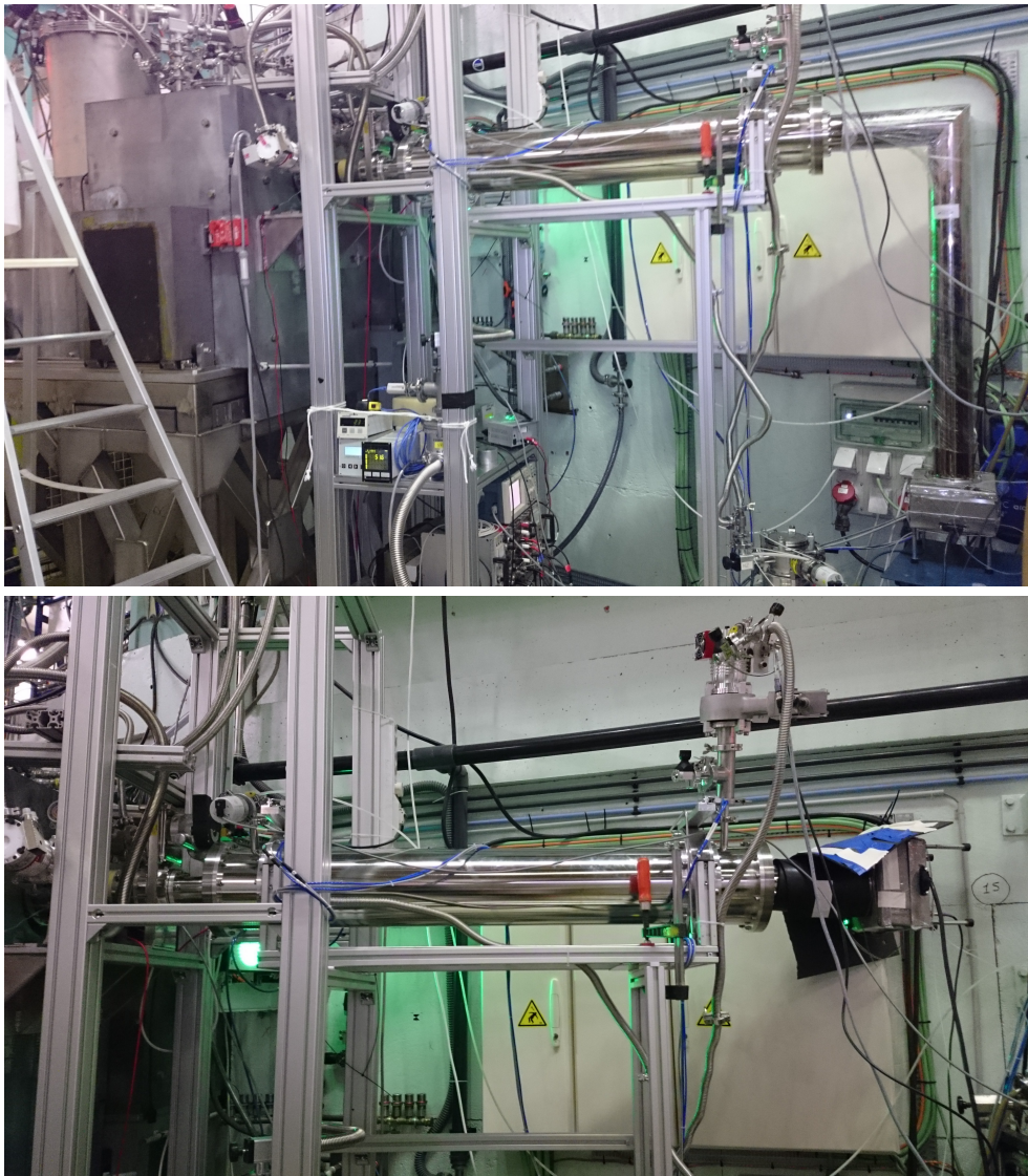
Figure 7.9: Photos of the setup installed at the SUN-2 source. Top: Vertical extraction, bottom: horizontal extraction.
