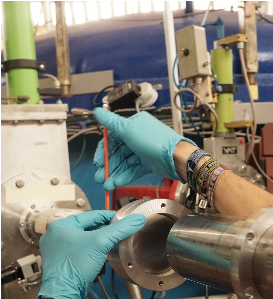
Figure 7.17: Top: Photos of the setup at turbine exit height at PF 2 , vertical extraction into the detector. The TEST beamline can be seen on the bottom right hand side. Bottom: Unmounting the vacuum safety foil. The blue turbine housing can be seen in the background.
