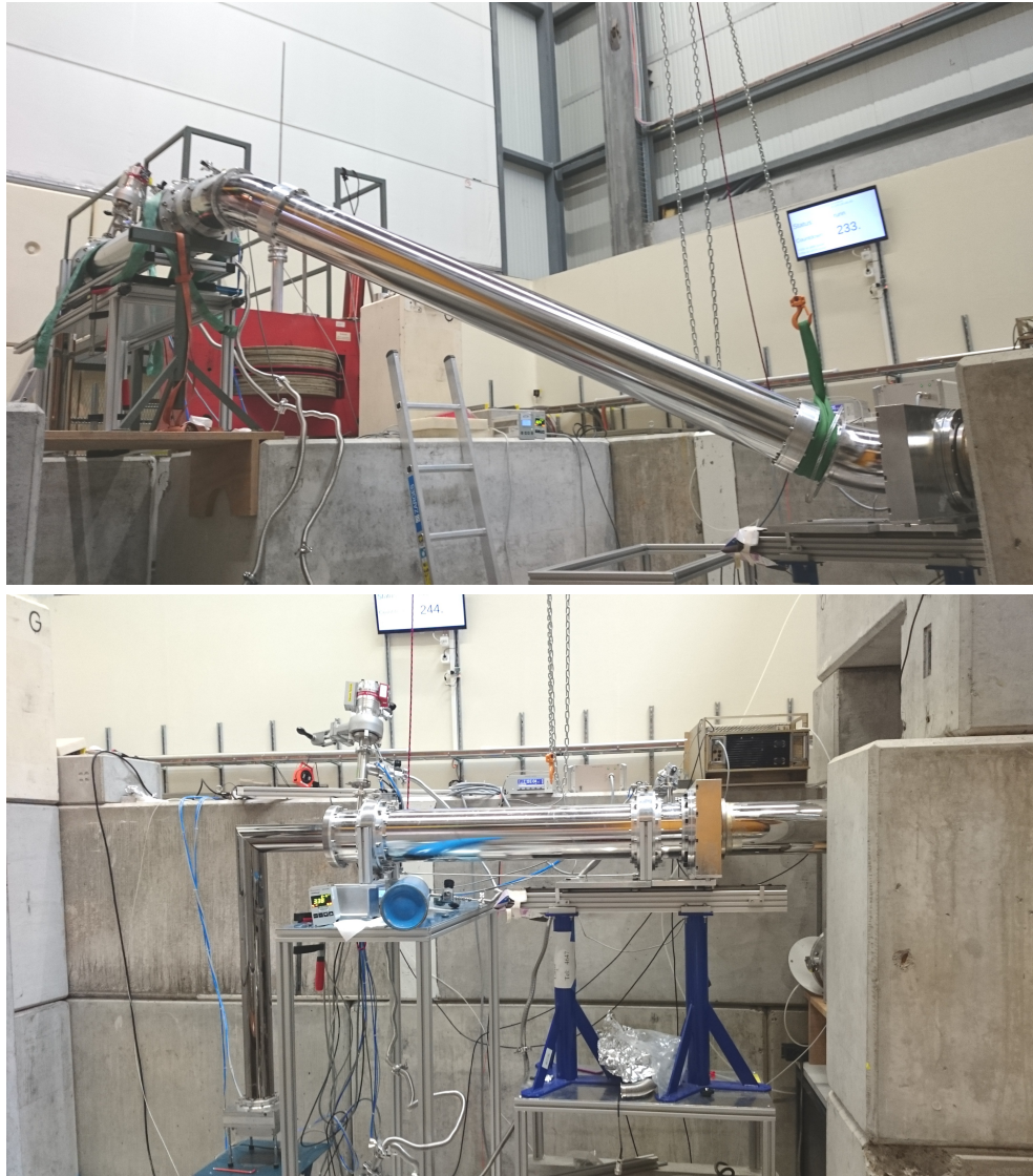
Figure 3.22: Setup at the West-1 beamport. Top: Storagebottle elevated by 1200 mm. Bottom: Storage bottle at the height of the beam port, without the 2 m guide and bends in order to measure calibration data needed to determine the transmission of the S-shaped beam line.
