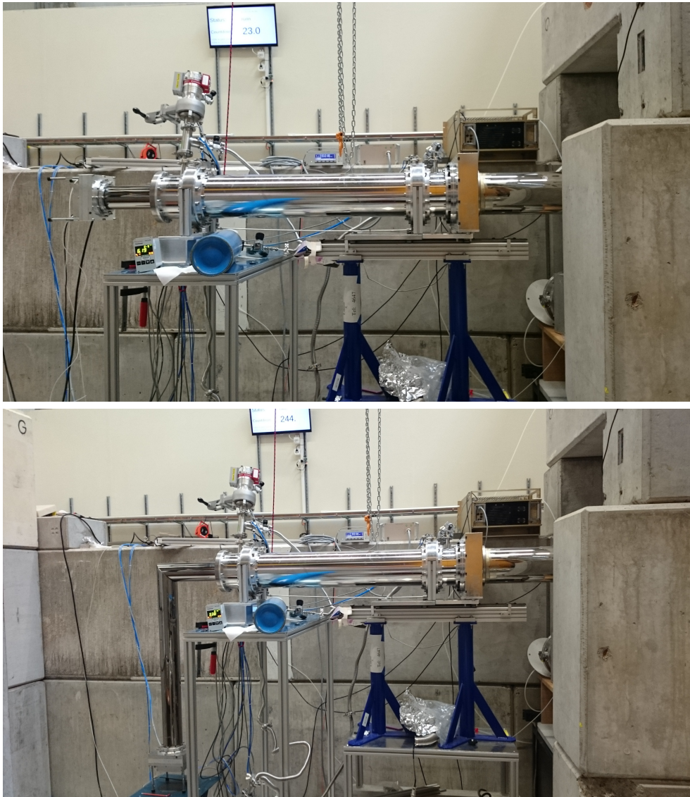
Figure 7.27: Setup at the West-1 beamport at the PSI UCN source. Top: Setup with horizontal extraction. Bottom: Vertical extraction.
