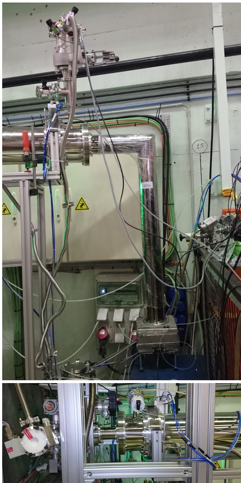
Figure 7.10: Details of the setup at SUN-2: Top: The vertical extraction guide plus detector. Bottom: Connection of the storage bottle to the UCN source.
