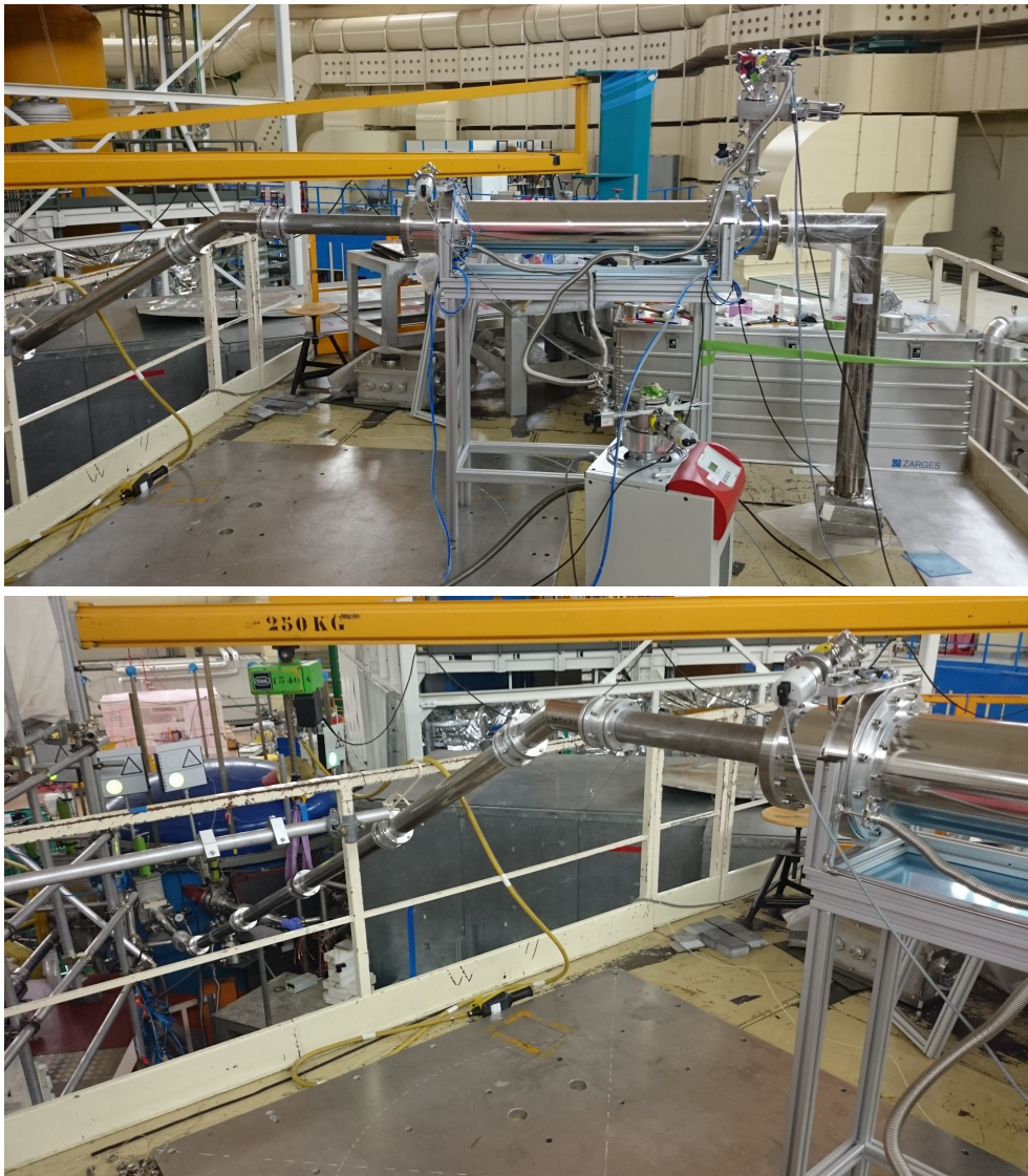
Figure 7.15: Photos of the setup on the EDM platform at PF 2 . Top: Storage bottle setup with vertical extraction. Bottom: UCN beamline up to the platform.
