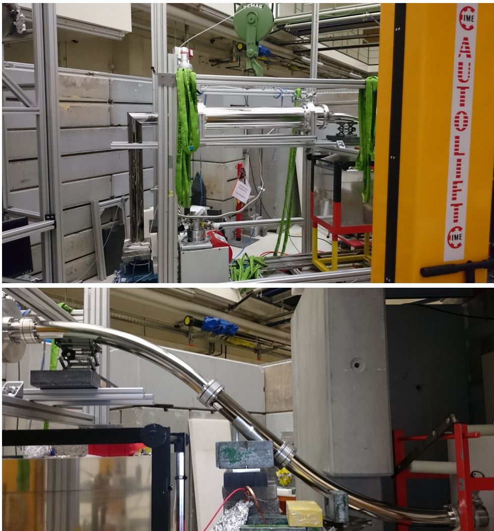
Figure 7.23: Photos of the setup at the TRIGA Mainz, beamport D. Top: Storage bottle setup with vertical extraction. Bottom: Beamline from the source port upwards to the storage bottle, shorter straight guide than in the final measurement.
