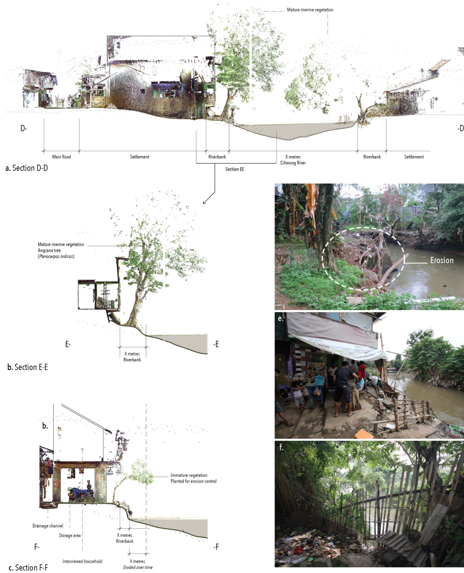
Figure 5.2.6: Terrain: a. Sectional elevation A-A ‘NGO’ provides an illustration of the height difference between the main street within the Bukit Duri neighbourhood and the river. Homes along the river are typically multi-level which helps households cope with recurrent flooding. b. and c. Sectional elevations B-B and C-C illustrate the role of mature vegetation within the river corridor in stabilising the riverbanks. Various examples of local strategies are visible within the neighbourhoods, including d. hard-edges such as rock and concrete, e. bamboo and timber planks, f. fencing.
