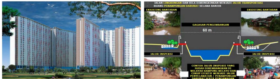
Figure 4.5.7: The normalisation of the Ciliwung River, among others, under the Jakarta Urgent Flood Mitigation Project has been underway since 2012 and includes river widening and dredging, the implementation of a service road, and requires resettlement of communities living within the demarcated river zone. Source: Kementerian Pekerjaan Umum, Daerah Khusus Ibukota Jakarta and Kementerian Perumahan Rakyat 2011.
