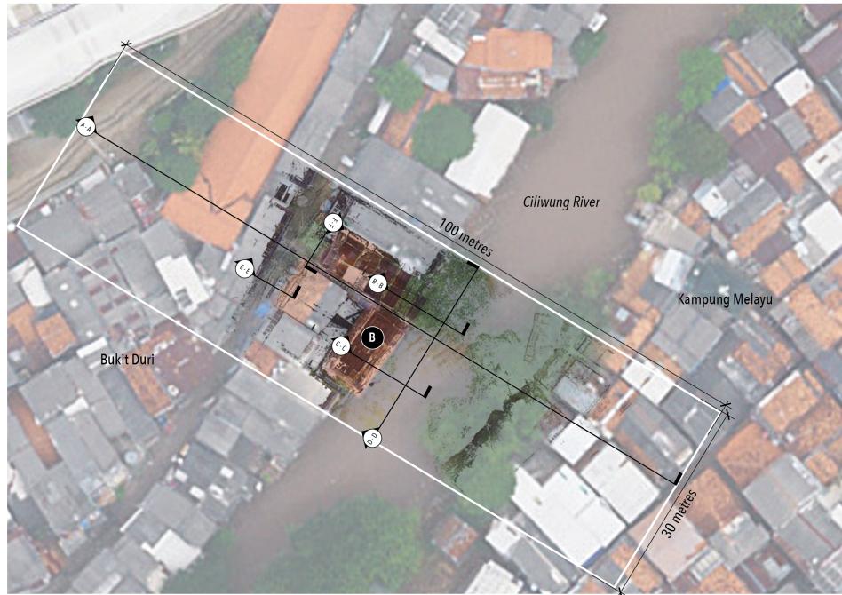
Figure 5.1.7: Aerial photograph (FCL) with overlaid terrestrial laser scan model of the 100x30 metre transect taken in Bukit Duri. A series of sectional elevations (A-A to F-F) were taken through the point cloud using Autodesk Revit. 'B' denotes one of the households specifically referred to within this chapter [193].
