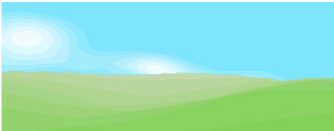
Figure 2.1.: Example of a Cosmocam image combined with the model topography. Light blue to white shows the integrated cloud water content (increasing from light blue to white) and green indicates topography (the further away, the lighter the green). The picture mode used to produce this Cosmocam data and corresponding image is 'integrated'.
