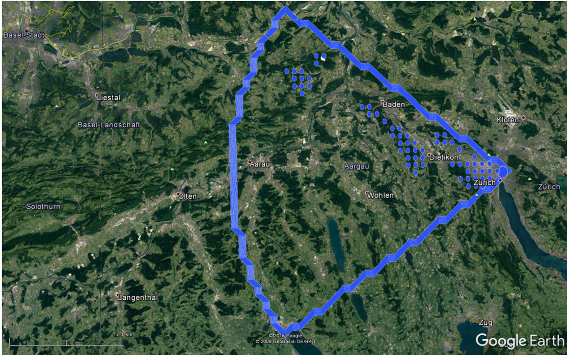
Figure 3.13.: Visibility map ' Frontal Passage '. The large blue dot represents the camera position and the small dots the visible COSMO 1 surface grid points within the marked field of view.
