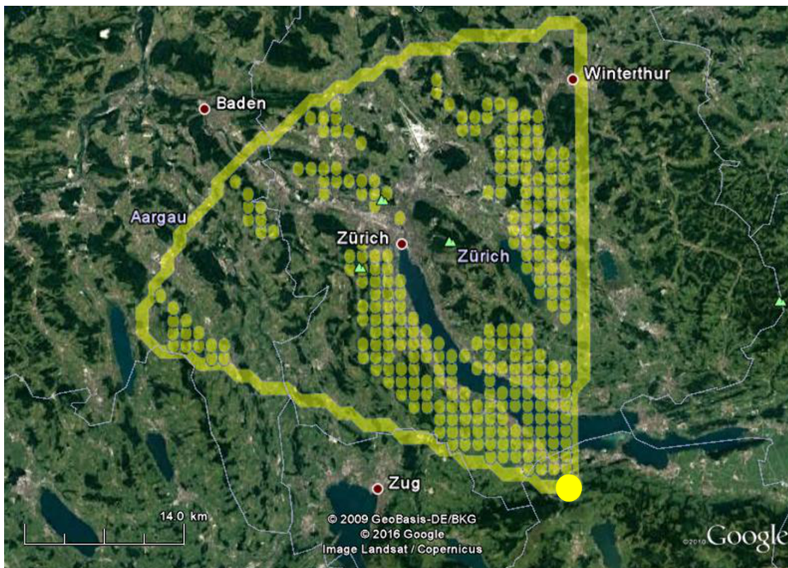
Figure 3.2.: Visibility map corresponding to the movie 'Seiche Lake Zurich' . The large yellow dot represents the camera position and the small yellow dots the visible COSMO 1 surface grid points within the field of view resulting from the Cosmocam parameters.
