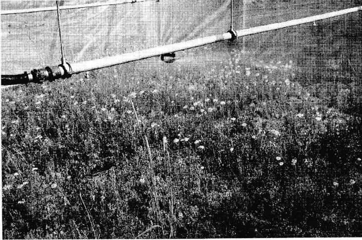
Figure 6.5 Model roof A during the conduction of the artificial rain event experiment.
