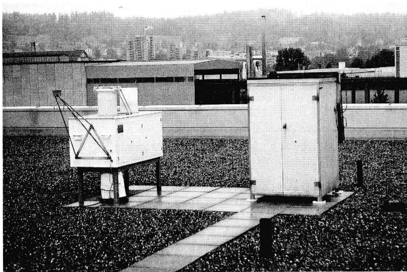
Figure 4.1 Bulk rain sampler (right) as used in Dübendorf, Grüze, and Tüffenwies.
