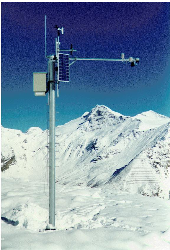
**Fig. 1b - Example of IMIS snow station.** Visible are among others the wind sensor on top and the ultrasonic snow depth sensor and the humidity / temperature sensor on the beam.
