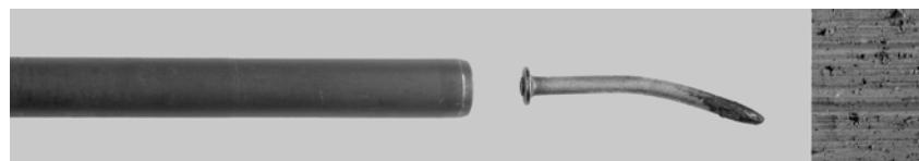
**Fig. 6 - Buckled nail on concrete**
