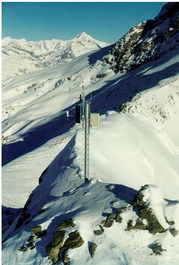
**Fig. 1a** - Example of IMIS wind station on a mountain crest. Visible are the solar panel, the logger-transmission box and some sensors.
