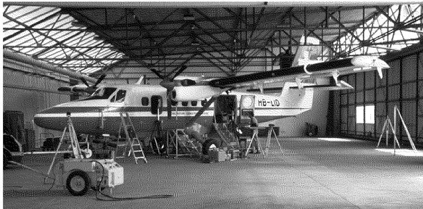
Figure 5.2.: Jacked up aircraft during the lever arms measurements.
