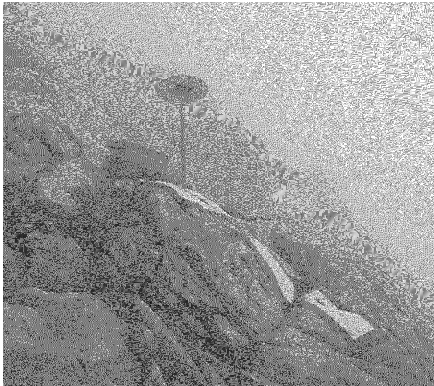
Figure 7.3.: Occupation of tripod 102 next to control point 3010 with a dual frequency GPS receiver.
