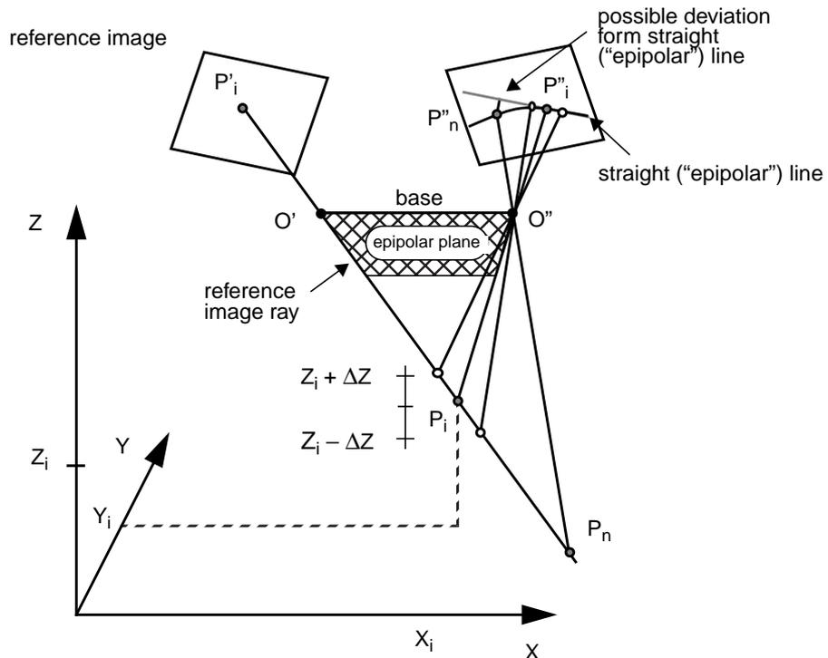
Figure 3 Approximation of epipolar geometry for SPOT images
