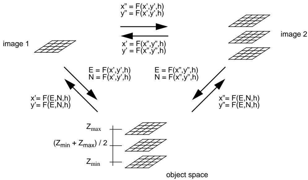
Figure 2 Derivation of fast polynomial mapping functions
