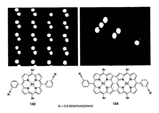
The first scanning tunneling microscopy studies on monolayers of triply linked and monomeric porphyrins show that 134 and 142 self-organize into ordered molecular bilayers upon co-deposition with  $C_{60}$ . The arrangement of the fullerene molecules on the patterned layer can be controlled by the porphyrin structure. The observed mode of self-assembly is
