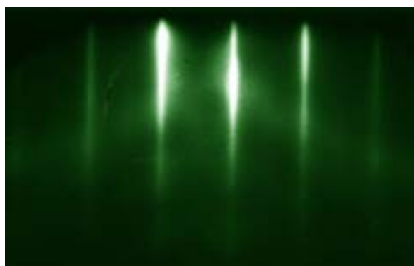
Fig. 3.24. Smooth surface RHEED patterns of \text{Pb}_{0.9}\text{Eu}_{0.1}\text{Se}/\text{BaF}_2/\text{CaF}_2/\text{Si} (100) ([011] azimuth).
