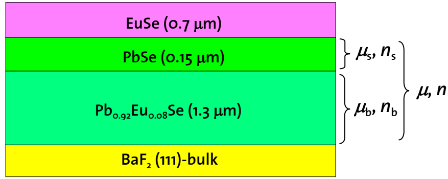
Fig. 5.2. Cross-section of the laser double heterostructure with PbSe active layer.
