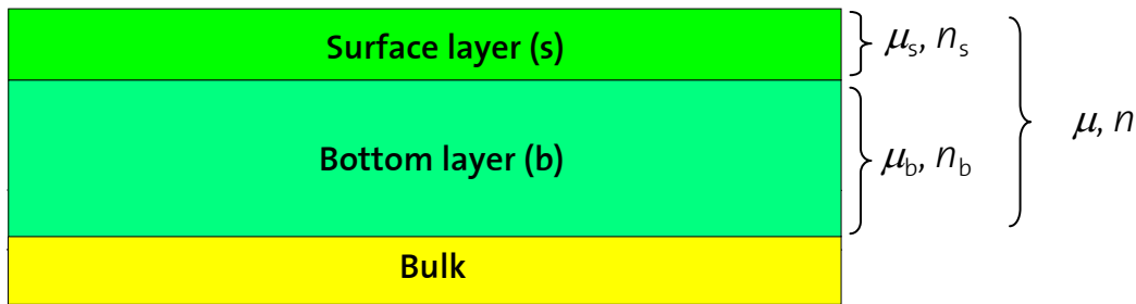
Fig. 3.29. Schematic cross-section of the structure with 3 layers.
