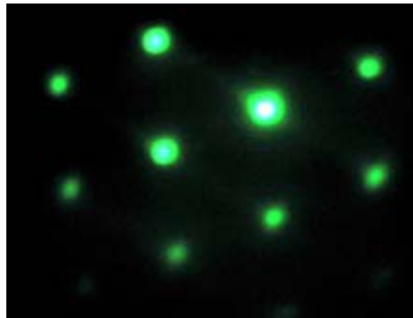
Fig. 3.12. EuSe on \text{Pb}_{0.95}\text{Eu}_{0.05}\text{Se}/\text{BaF}_2(111) RHEED image ( [-110] azimuth).
