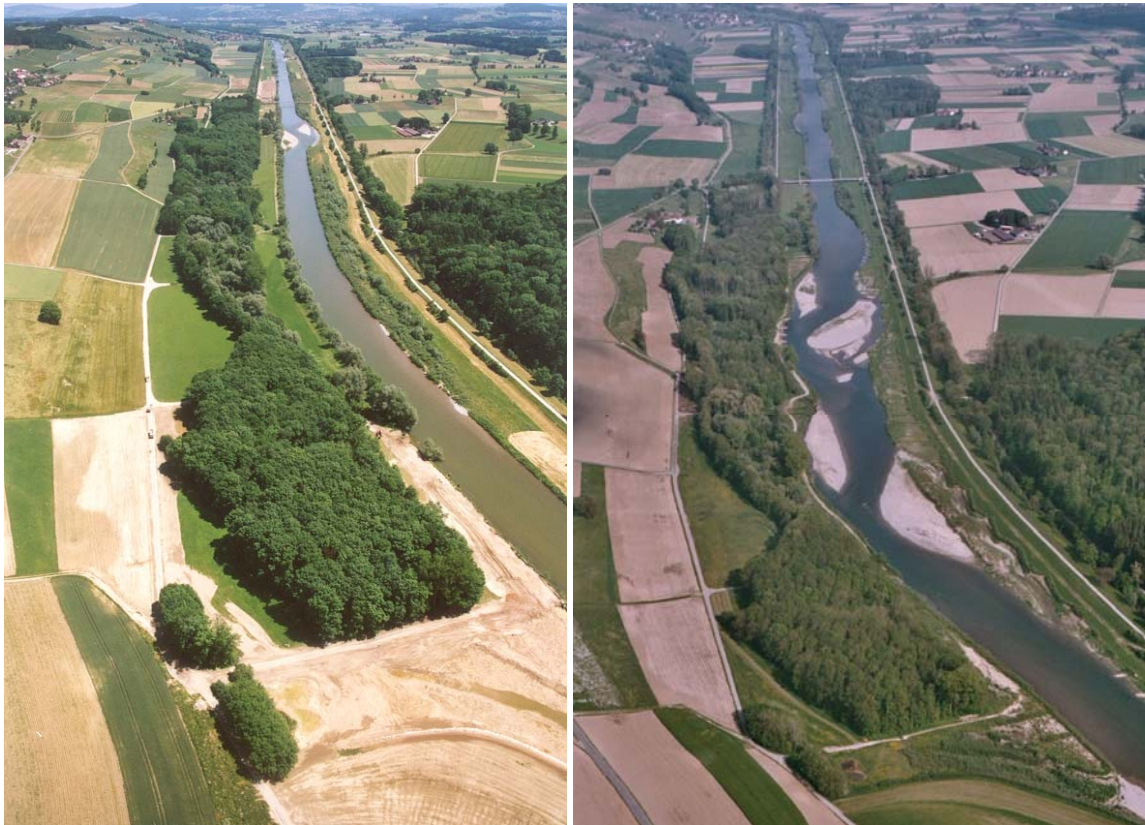
Figure 1.2: The Thur River, Switzerland, at Schafftäuli. Left: before rehabilitation in June 2001. Right: after rehabilitation in May 2004 (Photos by C. Herrmann, BHAtteam, Frauenfeld).
